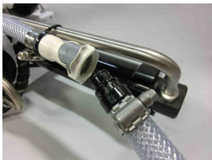
Connecting brine discharge service hose
