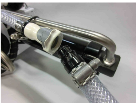
Connecting brine discharge service hose
