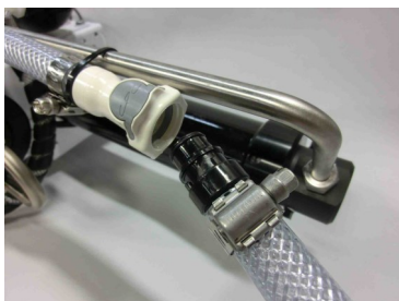
Connecting brine discharge service hose
