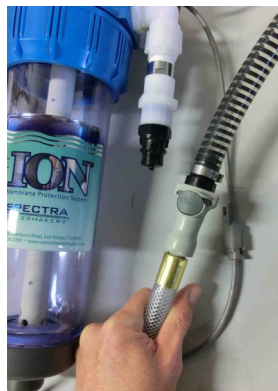
Replacing fresh water flush hose with intake service hose
